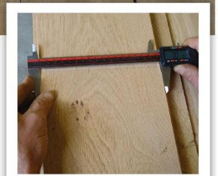
MC readings of kiln-dried flooring blanks preparing to be redried to 5 to 6 percent. Remember to take width measurements in the middle of flooring planks, as well as the ends.
