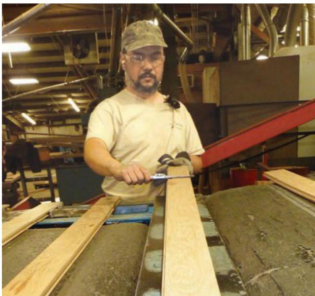
Mill Foreman Phillip Garcia does a quality check on White Oak flooring.
