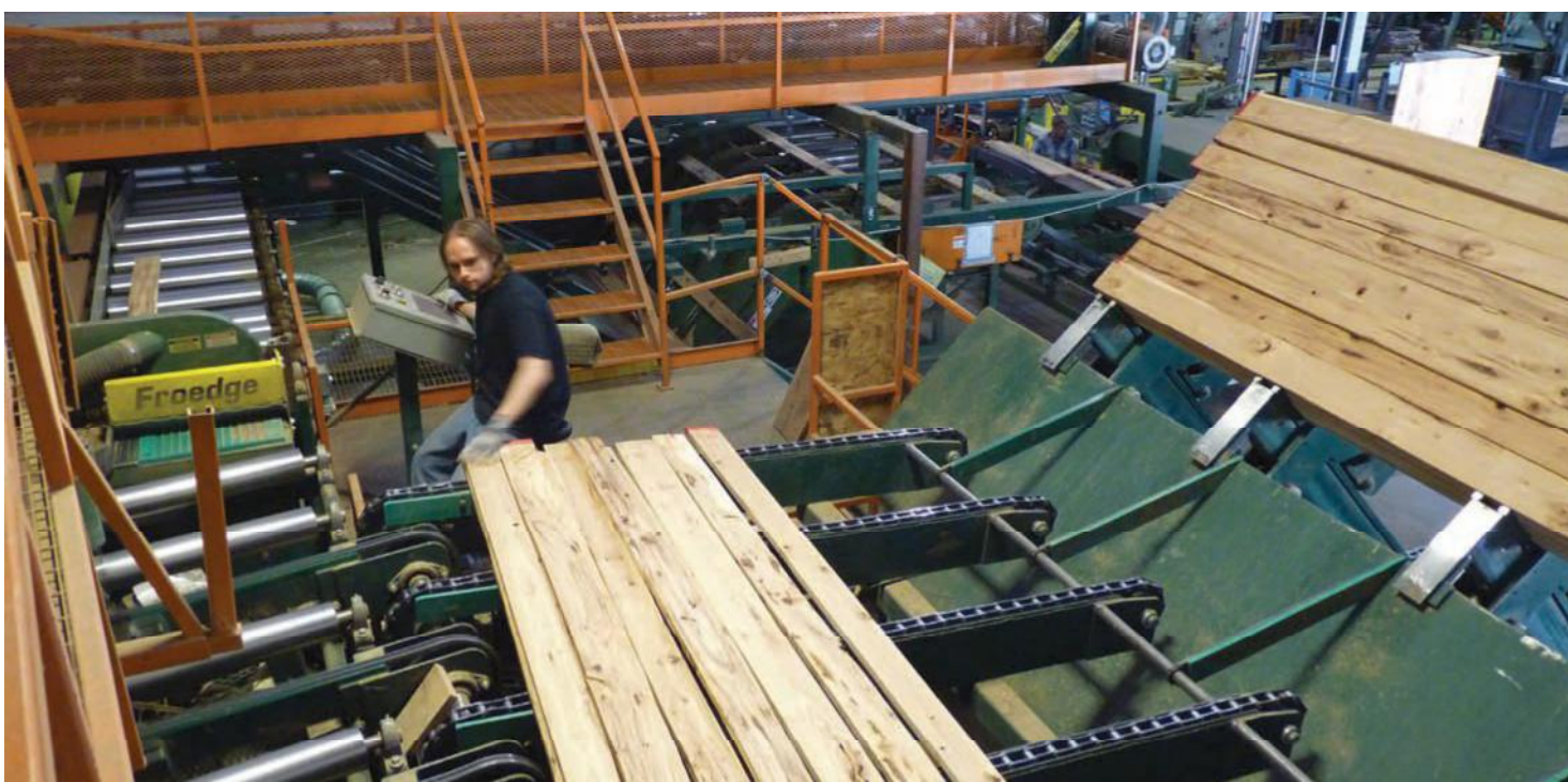
Muscanell Millworks, Cortez, CO, purchases over 3 million board feet of lumber annually to produce high quality Hardwood flooring. Pictured is a Muscanell team member overseeing the lumber infeed to the rip saw.
